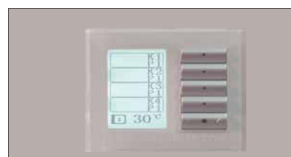
Home automation - 8-in-1 sensor Section 9 (Utilities)
