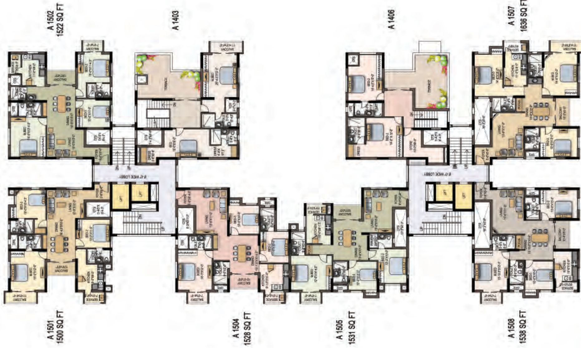
PHASE 1 BLOCK A - 3 BED UNIT FIFTEENTH FLOOR PLAN DUPLEX AND TYPICAL FLOOR PLAN
